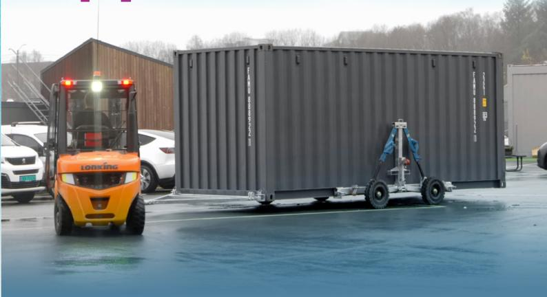
Norwegian equipment supplier Wee. no has launched ContainerWheels 2-in-1, a patented system designed to make container transport more flexible. The system allows for lifting and towing containers, slashing the need for heavy machinery or permanent infrastructure.
